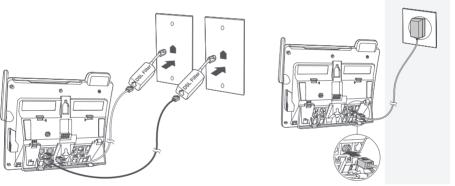
4. Align the mounting studs on the mounting plate with the mounting holes on the bracket and press the telephone base down until it clicks securely into place.
