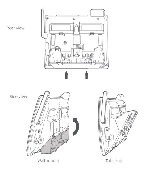
4. Plug the telephone line cord (or DSL filter) into the wall jack. Plug the power adapter into an electrical outlet not controlled by a wall switch. Bundle the telephone line cord and power adapter cord neatly with twist ties, if necessary.
