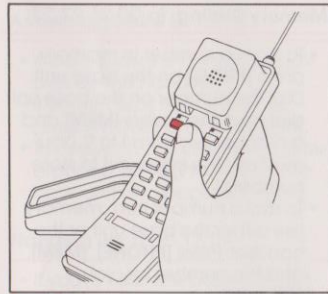
Figure 1: To make a call on the handset, press [PHONE] , then dial the number.
